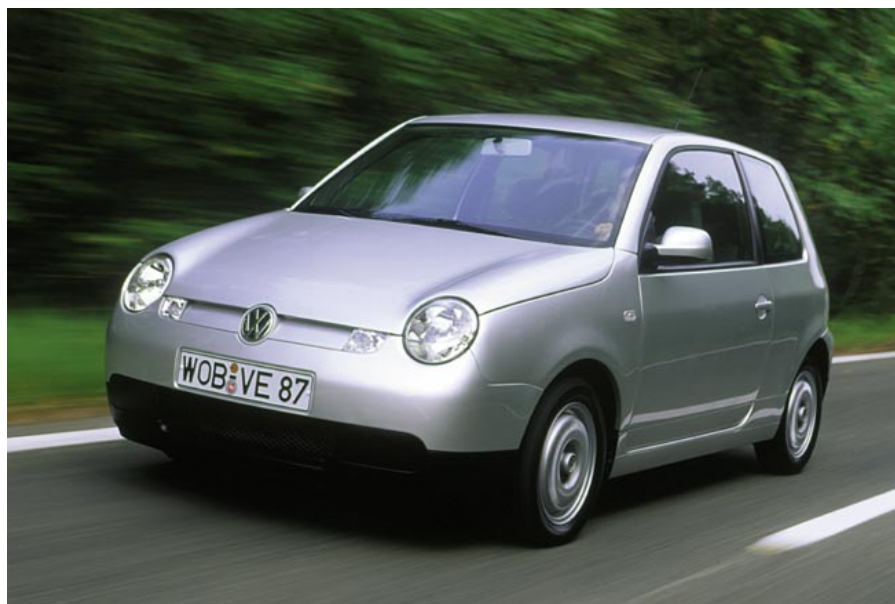
More energy-efficient vehicles are a key element in the alternative energy scenario, Carbon 15. The diesel version of the Volkswagen Lupo, with a fuel consumption of only 3 litre per 100 kilometres, is an example of progress in this direction.
