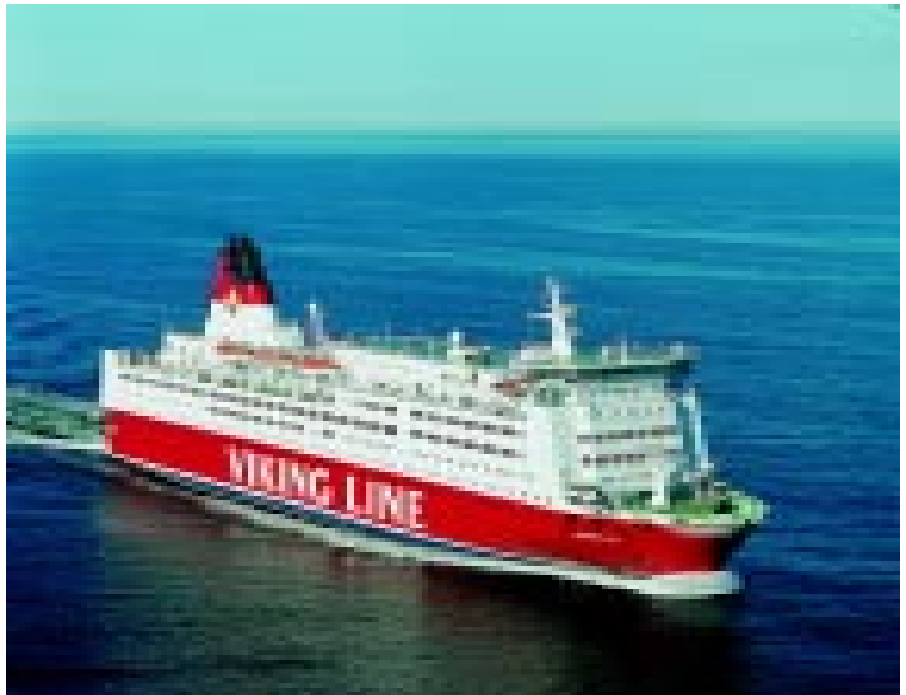
Viking Line's MV Mariella is the first passenger ship in the world to use HAM technology on all its main engines. The technology has reduced emissions of nitrogen oxides by 80–85 per cent.
