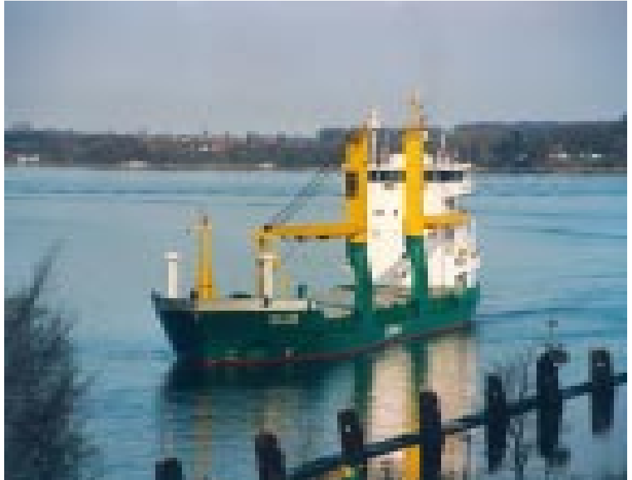
The freighter MS Cellus emits 90 per cent less nitrogen oxides and 80 per cent less sulphur dioxide than an equivalent standard ship. It is equipped with an SCR flue gas emission control system and uses low-sulphur fuel oil.
