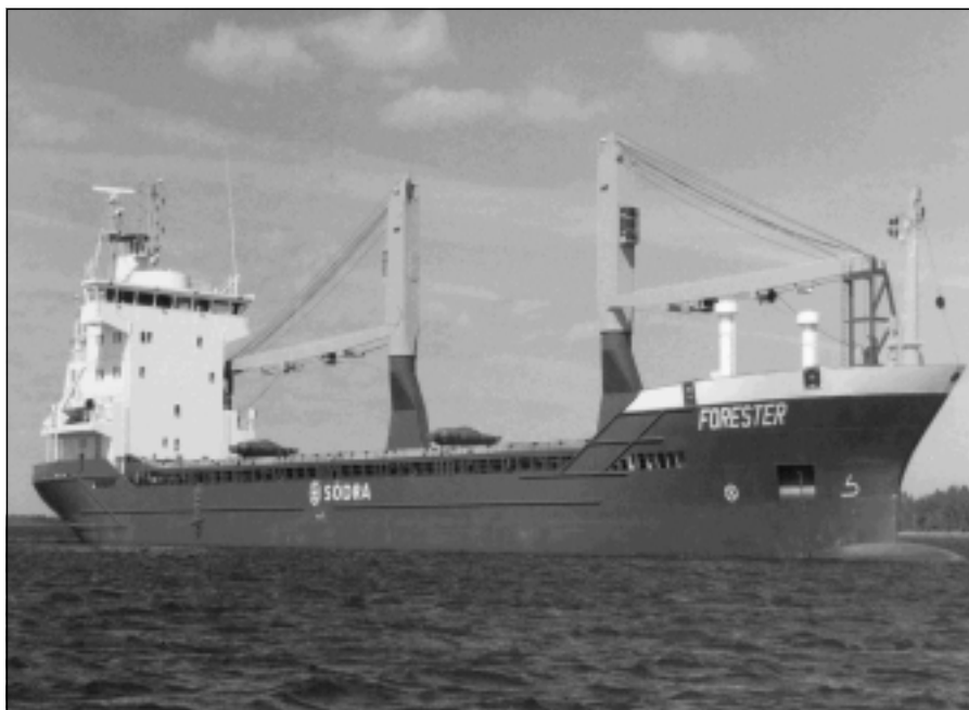
Three vessels used by the Swedish forest-products company Södra run on low-sulphur oil and are equipped for catalytic cleaning of the exhaust gases. There are no technical reasons for not cutting down the emissions of air pollutants from shipping.
