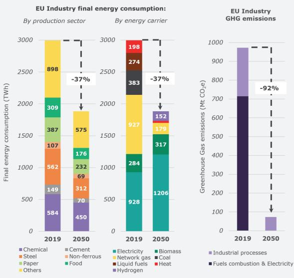
The diagram on the left represents the evolution of energy carriers in EU27 industry. The transformation of the industry from a high-carbon industry to a low-carbon industry reduces its FEC by 34%. This transformation relies mainly on renewable electricity and – to a lesser extent – on biomass, renewable gas and hydrogen associated with steel production via HDRI.
